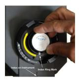
The provided indexing ring is then placed on the standard facing forward toward the index mark on top of the MTOL+.
