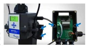
Next, mount the base portion on top of the junction box. The recommended mounting hardware is M6 or ¼" screws. Four screws are needed.
