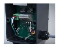
All electrical connections are made inside the junction box. Choose the appropriate cable gland for each connection. Any modifications to the junction box could affect the warranty.
